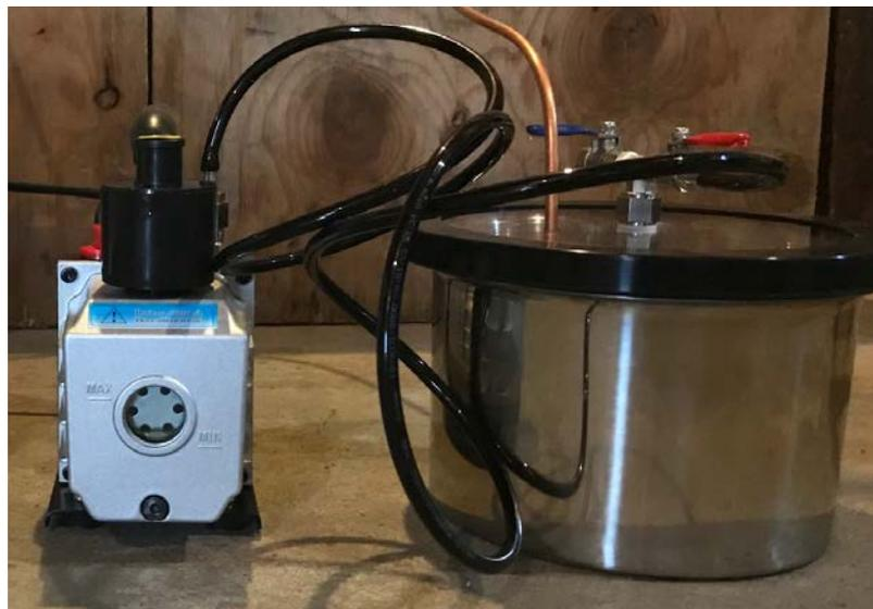
Figure 6: Vacuum Pump and Moisture Knock-Out
