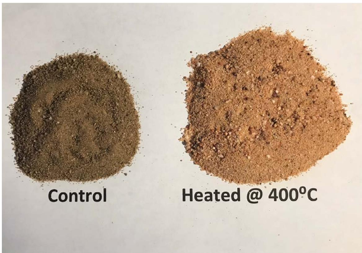
Figure 7: Soil before and after thermal treatment
