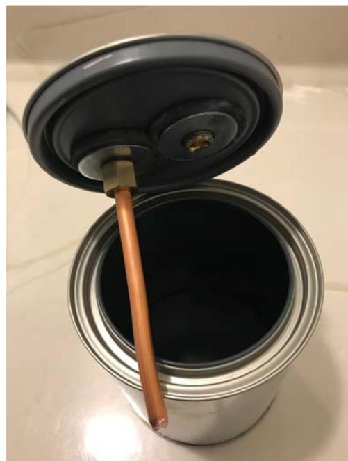
**Figure 4: Air Inlet Tubing**
